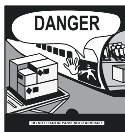
Handling Label for Cargo Aircraft Only, reduced size, black on orange
